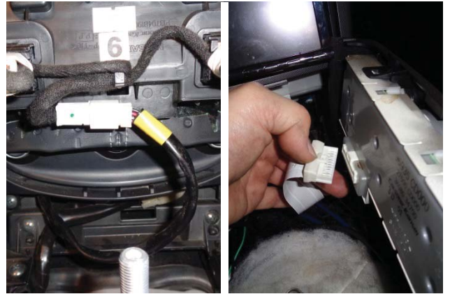
8. Disconnect all electrical connectors, and remove the shifter panel from the vehicle.
