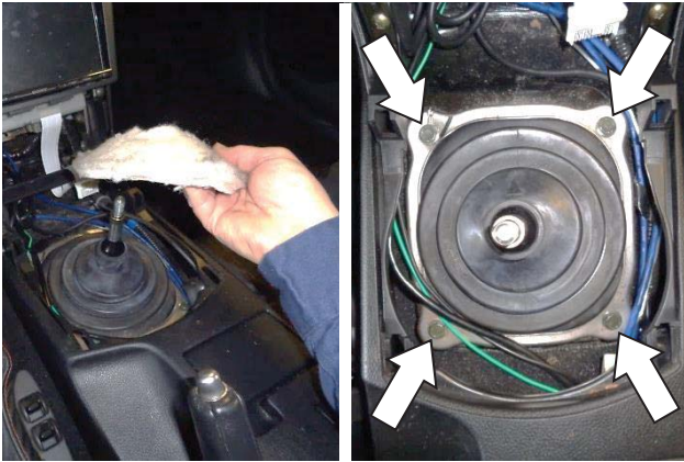
11. On 350Z and similar: Lift the insulating pad over the shift lever. Then remove and retain the 4 screws from the outer dust boot and metal frame.
