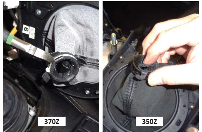
9. Remove the plastic ring from the leather boot. Some models (370Z and similar) require cutting a cable tie. Use care to avoid tearing the leather.
