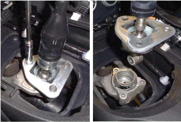
17. CAUTION: SHIFTER PLATE IS UNDER SPRING TENSION. Carefully remove the 3 shifter plate screws, then remove the shifter and plate. Retain the shifter plate for re-use.
