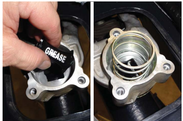
21. Apply a thin layer of grease (10) to the bottom and sides of the shifter housing. Then reinstall the spring.
