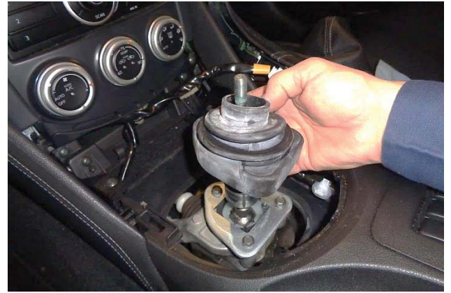
14. Pull the inner dust boot off of the shifter plate and lift it over the shift lever.
