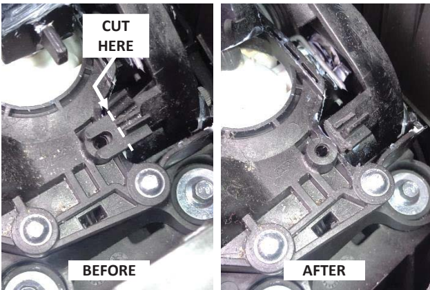
26. With a utility knife or diagonal-cutting pliers, cut the two lobes off the alignment notch as shown.
