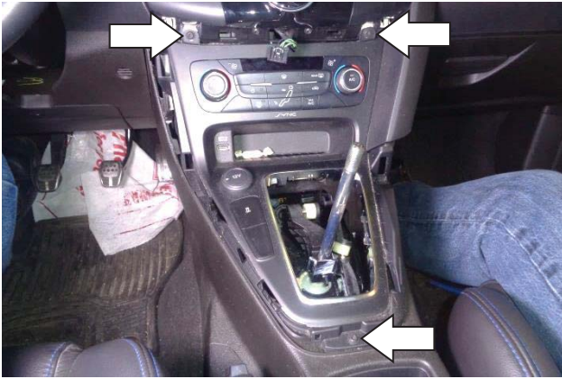
19. Remove the 3 power panel screws.
