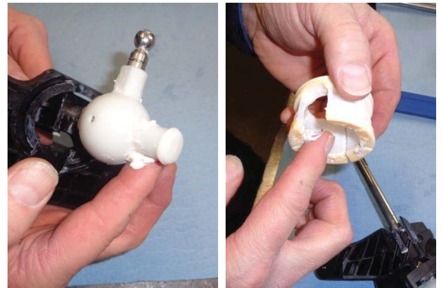
35. Temporarily transfer any grease from the main and side pivot balls into the main pivot cup (to be used later).
