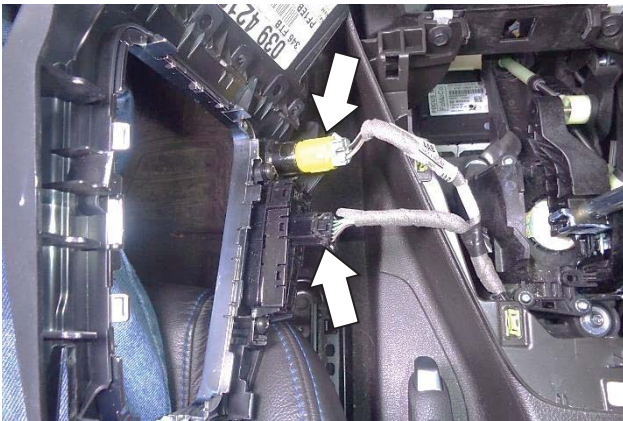
57. Reconnect the yellow (12V) and black (traction control) connectors.
