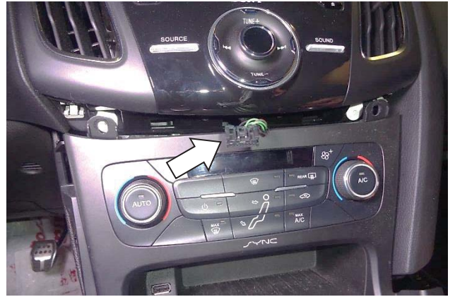
59. Ensure that the center panel bezel plug is exposed and accessible before reinstalling the power panel.
