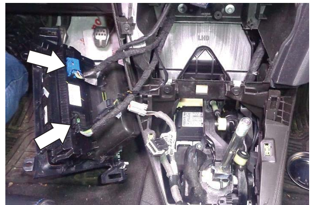
24. Disconnect the blue (AUTO) and black (AC) connectors, and remove the power panel from the vehicle.
