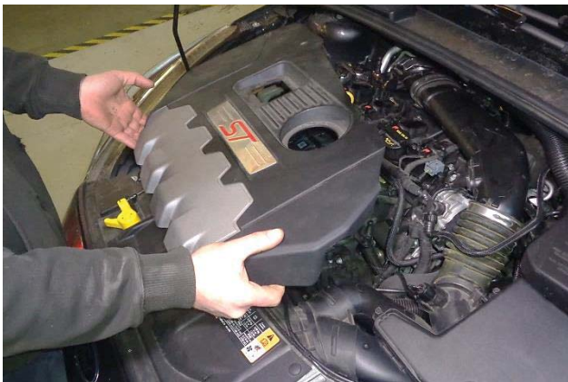
82. Install the engine appearance cover.
