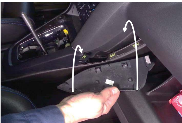
64. Open the glove box, reinstall the console side panel, then close the glove box.
