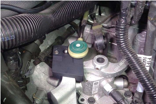
44. Snap the cable end onto the ball stud.
