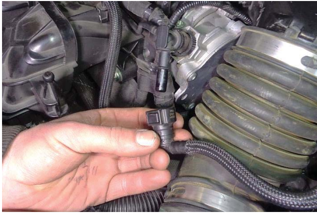
80. Connect the breather hose to its fitting.
