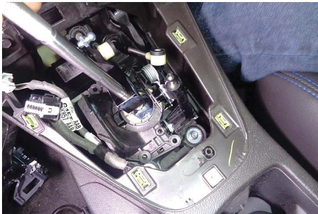
50. While holding the spring open, install the shift lever by inserting the pivot cups into their respective openings. Then gently release the spring end into the groove on the grommet, and move the shifter top housing into place on the bottom housing.
