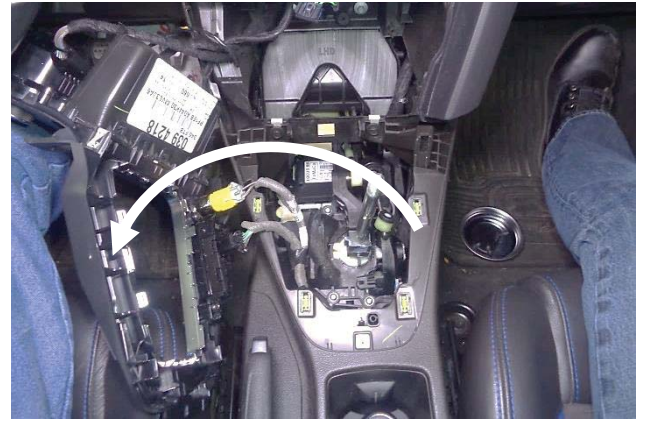
22. Carefully flip the panel toward the left, taking care not to strain the 4 electrical connectors.
