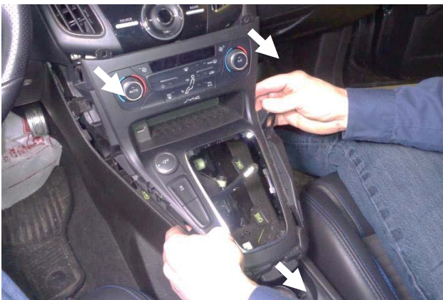
21. Pull the panel rearward to clear the center dashboard.
