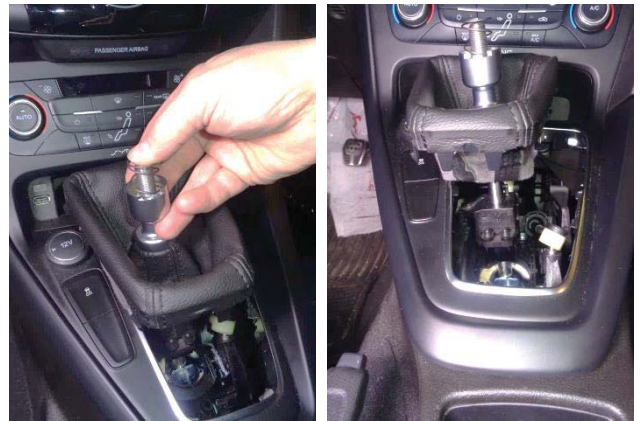
66. Move the shift lever into REVERSE gear.
