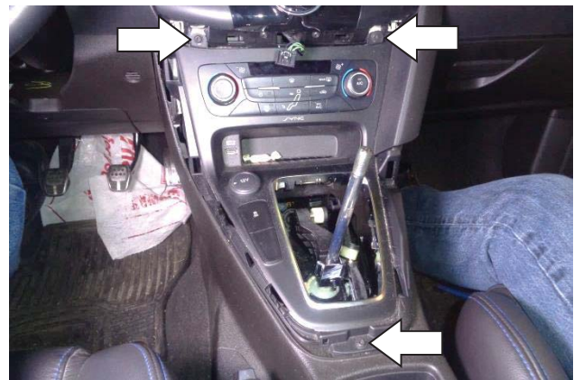
61. Install and tighten the 3 power panel screws.
