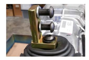
15. Installation is complete and ready to place into the vehicle. This shifter locates the handle in nearly the same location as the stock shifter hole in the floor. There may be some modification required to the floor or tunnel area to accommodate the larger size of the Tremec transmission.
