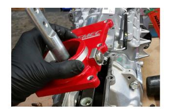
6. Use rubber mallet to jar cover plate loose and remove.
