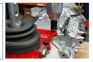
Remove the rubber boot from the original Tremec shifter
