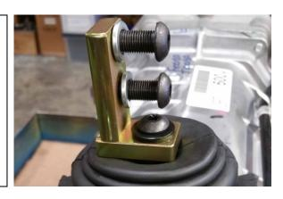
Attach the Chrome Hurst shift handle to the lower stub stick using the supplied hardware. Reinstall the shift boot and factory console. If you are using a properly designed crossmember and your car is in good condition (no floor sag, stock height sub-frame mounts that are not worn, and properly aligned sub-frame), there will be no modifications required to your floorboard or console when using this shifter.
