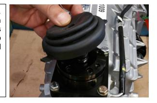
Position the offset stub onto the shifter and make sure that it is offset towards the driver's side as seen in the photo. Secure the offset stick with the provided 3/8"-24 Button Head bolt and washer and torque to 35 ft/lbs.
