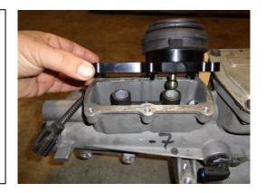
When you are sure your shifter is correctly positioned, apply a new bead of RTV sealer to the lip of the shifter cavity and mount the shifter by re-using the six, 5/16" bolts. Torque the bolts to 20 ft/lbs.
