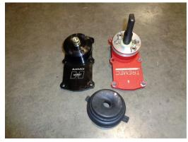
Install the modified boot onto the Blackjack shifter. Confirm that the rubber boot does not interfere with shifter movement and that the shifter lever movement is not restricted or binding at full travel positions. Failing to do so could result in the shifter popping out of gear and damaging the transmission.
