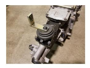
Attach the Chrome Hurst shift handle to the lower stub stick using the supplied hardware. This shifter locates the handle in nearly the same location as the stock shifter hole in the floor. There may be some modification required to the floor or tunnel area to accommodate the larger size of the Tremec transmission.
