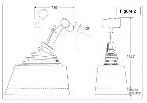
3. Drill four 9/32" mounting holes where marked. Temporarily mount the shifter in place using washers as required to get it level. **Do not bend the mounting brackets on the bottom of the shifter.** Mark the location for the shifter cable hole, 3" ahead of the left front shifter mounting hole. Drill or cut a 1-1/2" diameter cable hole in the floorboard.
