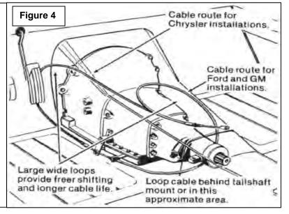
9. Seal the hole where the cable goes through the floorboards to prevent air or water leakage. A putty type sealer can be used. For General Motors vehicles go to Step 10, for Ford vehicles go to Step 15, for Chrysler vehicles go to Step 21.
