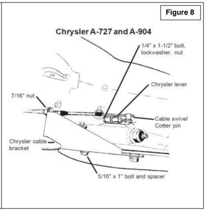
22. Remove the two transmission oil pan bolts directly below the shift lever. Install the cable bracket in position with the two spacers between the pan and the bracket (See Figure 8). (If your transmission is equipped with a cast aluminum oil pan these spacers can be omitted.) Install the two 5/16-18 x 1.00" pan bolts supplied and tighten to 12-13ft/lb. Do not overtighten as this can damage the pan gasket.
