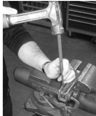
10. Tap the 2 roll pins through the selector plunger. Then flip the carrier over in the vise, and remove the pins.
