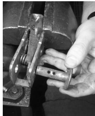
11. Remove the selector plunger and reverse plunger.
