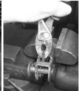
10. Tap the 2 roll pins through the selector plunger. Then flip the carrier over in the vise, and remove the pins.
