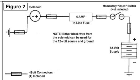
IMPORTANT: The solenoid must be energized for the shifter to remain in 1<sup>st</sup> gear.
