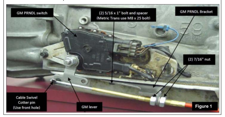
Step 2. The bracket must be installed with the two spacers between the pan and the bracket. (If your transmission is equipped with a cast aluminum oil pan, these spacers should be omitted. Install the two  $5/16-18 \times 1.00$ " bolts (Metric transmissions use the two 8mm x 25mm bolts) supplied and tighten 12-13 lb-ft. Do not overtighten as this can damage the pan gasket. (See Figure 2)
