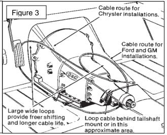
STEP 4. Move the transmission selector lever by hand to the full rear position (LOW). Place the shifter lever to the LOW gear position (all the way back). Adjust the large nuts on the cable so that the swivel will slide into the correct hole ("F" holes) on the selector lever. Tighten the large nuts completely. Be sure that the swivel will slide freely in and out of the hole in the selector lever. Note: The shifter will not operate correctly unless the correct hole in the selector lever for
