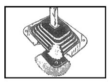
5. Slip bottom boot lip under carpet. Place hold-down plate into position and fasten with sheet metal screws supplied. Remove protective paper on chrome side of hold-down plate.
