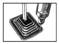
4. Replace boot. Drill 1/8" diameter holes through floor using boot holes to locate hole positions.
