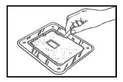
2. Remove the boot and place the chrome-plated retainer plate exactly within the traced outline. Trace the inside opening of the plate on the carpet with chalk.
