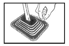
1. Remove knob. Slip boot over stick and down to floor. Use chalk to trace the outline of the boot on to the carpet.
