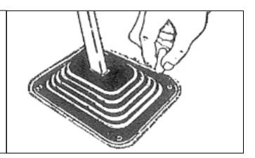
2. Remove the boot and place the chrome-plated retainer plate exactly within the traced outline. Trace the inside opening of the plate on the carpet with chalk.
