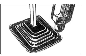
5. Slip bottom boot lip under carpet. Place hold-down plate into position and fasten with sheet metal screws supplied. Remove protective paper on chrome side of hold-down plate.
