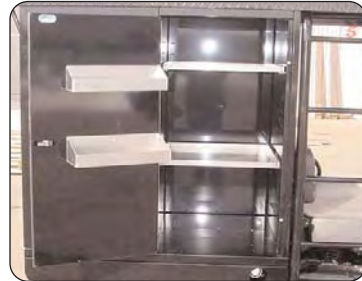
INSIDE OF CABINETS SHELF, RADIUS ROD HANGER, AND OIL CAN BINS
