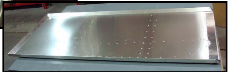
STEP #34 Rivet on (Item 40 & 41) Back Inner & Outer Corner Caps Check to see if all your Rivets are in Place! Your LH Board is now Complete!
