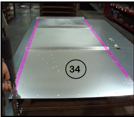
STEP #30 Rivet along Top & Bottom edge Note: Make sure to squeeze up on Wrap around lip!
