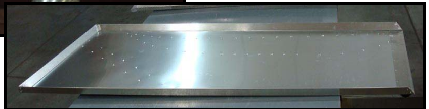
STEP #42 Rivet on (Item 40 & 41) Back Inner & Outer Corner Caps Check to see if all your Rivets are in Place! Your RH Board is now Complete!
