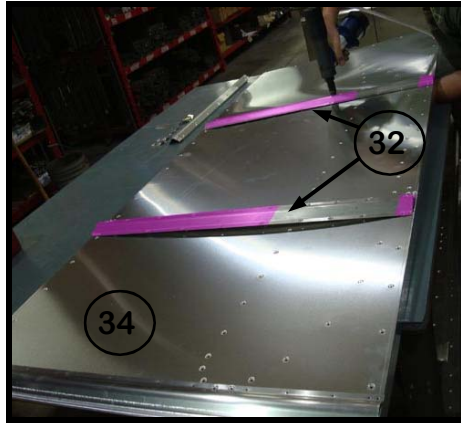
STEP #28 Rivet on 2 of (Item 32) Note: Make sure rivet protrudes thru all layers!
