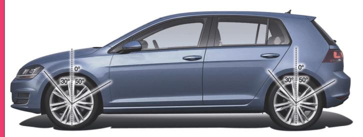
The overall width of the wheel arch must cover the tyre at least in the area limited by the radial planes 30° in front of and 50° behind the centre of the wheel.
