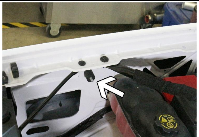
11. In the indicated area shown install the 8mm vibration mount and secure the mount with an 8mm nut and washer provided in hardware kit.
