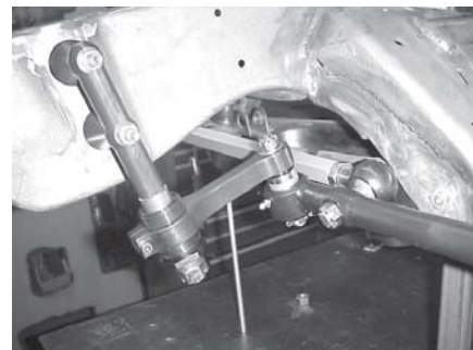
Howe Idler installed on a Chevelle reproduction frame with #32165 spacers.
