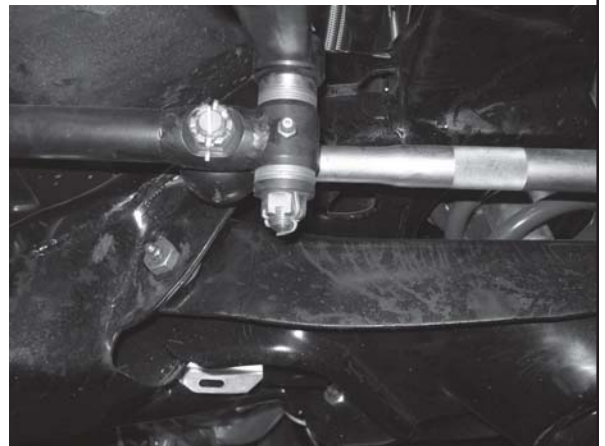
The height of the inner ends of the tie rods can be adjusted by moving shims on the Howe centerlink.
