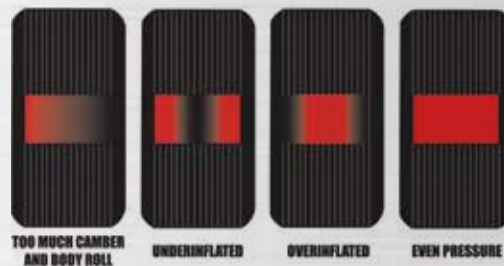
Each tire makes the most traction when the contact patch is equally loaded across its entire width. These illustrations show how the contact patch can be unequally loaded due to pressure or camber adjustments.
