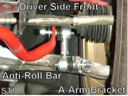
(Step 2) Use a 9/16" wrench and a 3/16" allen wrench to tighten the nylock nuts for each stud. (Tip: If possible, try using a "ratcheting wrench" to speed up the process.)
