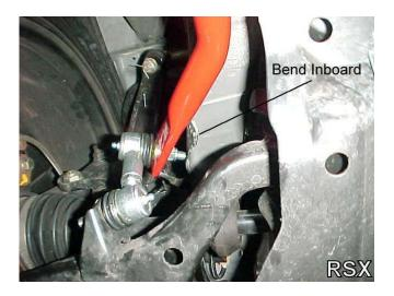
You are finished with the front end link installation! Make sure to re-check all hardware tightness after the first 100 miles, or if you hear a knocking sound from the front.
