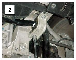
Once you disconnect everything pop the lower end link stud out of the holes, slide the bar sideways and twist it out of the vehicle.
