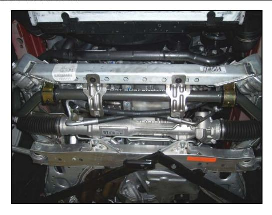
7F Reinstall Splash Guard Install splash guard and your done with the front.
