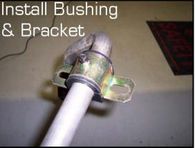
Apply a small amount of anti-seize to the threads of the U-bolts. Next position the axle bracket up against the axle tube. Raise the sway bar up to meet the axle bracket and allow the U-bolts to poke through the bushing bracket. Fasten the assembly together with the provided nut and washer. Do not fully tighten.
