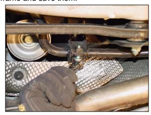
6/ As you begin to remove the bar, gently free each end from the end link sleeves. Now that the bar is free, slightly lower the exhaust by applying pressure to the tips just enough to remove the bar towards the front or the rear of the car.
