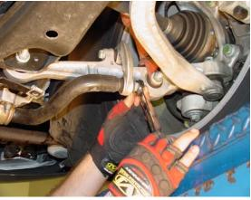
5/ Apply a quarter tube of grease to each inner-channeled portion of the two new front bushings and attach to Hotchkis bar against the outside of the washers on the bar. Slip the new brackets over the bushings.
