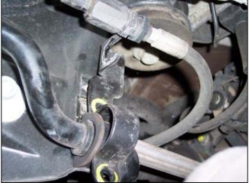
6) Remove the two end link bolts and nuts (16mm wrench) which attach the bar ends to the end links and save them. To clear the shocks with the bolts, pull the bar towards the rear of the car.
