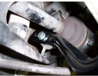
Adjustability Note: To adjust between the two holes, you must unbolt the bushing bracket bolts and pull the bar towards the rear so that the end link bolts clear the shock bodies. The hole at the bar's end is the normal setting, while the second hole from the end is the stiffer setting.
