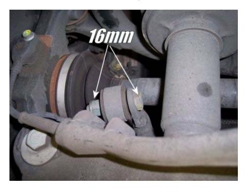
7) As you begin to remove the bar, gently free each end from the end link. Now that the bar is free, you can snake the sway bar through the exhaust pipes.
