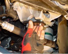
7/ Re-install the bracket nuts and tighten. <u>Use a small portion of blue thread-locker on the end-link bolts</u>, re-install and tighten well. \*\*Note\*\* If vehicle is raised using jack stands or other, the bar end and the end link may not align properly. Lower vehicle so that front suspension is not at full droop and ends will align. <u>Be sure to thread end link bolt by hand at first to prevent cross threading</u>.
