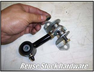
7) Again using the stock hardware, install the end links to the cast suspension arms making sure the lower grease fitting points towards the rear of the car.
