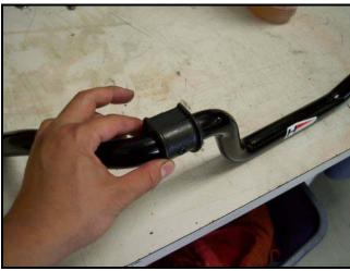
6) Lift the bar up to the vehicle. The two smaller H-Sport Stickers at the bar's end's should be right-sideup. As you lift the bar to the mounting points, you must place one spacer plate per side between the bushing and the mounting point. This relocates the bushing out of the stock bushing pocket.
