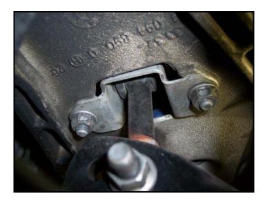
4) Remove the stock bushing brackets on both the driver and passenger sides.
