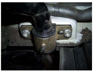
7) Re-install the bracket nuts and tighten. Then re-install the end link ends and nuts on one of the three available adjustment holes. We suggest the softer adjustment or the holes at the bar's ends.
