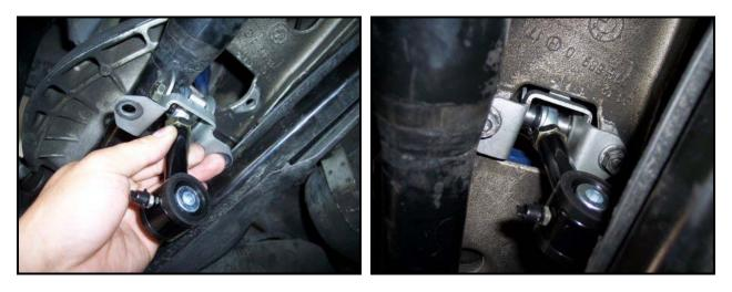
9) Apply grease along the inside surface of your polyurethane bushings. Install the rear bushings onto the bar at the approximate mounting location. Now you may install the H-Sport rear bar with the H-Sport sticker facing the rear, right side up.
