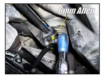
5) The stock rear bar is now free and can be removed as shown below. If you are having clearance problems, may have to remove the bushings and brackets or even twist the end links forward to remove the bar.
