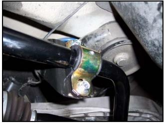
11) Attach the end links to the bar ends (inner hole for more roll resistance and the outer hole {near the ends} for less roll resistance) using the 10mm bolts, nylock nuts and small and large washer. Use the large diameter washer to capture the outboard side of the end link bushing and the smaller washer for the inboard side against the sway bar end.
