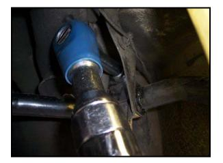
5) The stock rear bar is now free and can be removed as shown below. If you are having clearance problems, you may have to remove the bushings and brackets or even twist the end links forward to remove the bar.
