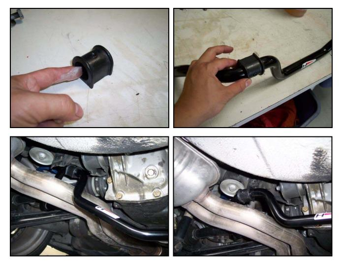
10) Next, slide the bushing brackets over the bushings. Position the bracket onto the stock mounting point. You will need to install the provided aluminum reinforcement plate on the backside of the mount. Fasten the bushing bracket and reinforcement plate together using the provided hardware.
