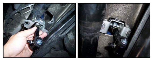
9) Apply grease along the inside surface of your polyurethane bushings. Install the rear bushings onto the bar at the approximate mounting location. Now you may install the Hotchkis rear bar with the H-Sport sticker facing the rear, right side up.
