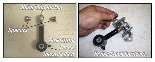
7) Again using the stock hardware, install the end links to the cast suspension arms making sure the lower grease fitting points towards the rear of the car.
