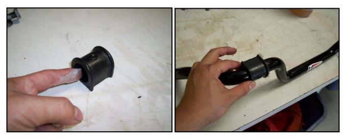
6) Lift the bar up to the vehicle. The two smaller H-Sport Stickers at the bar's end's should be right-sideup. As you lift the bar to the mounting points, you must place one spacer plate per side between the bushing and the mounting point. This relocates the bushing out of the stock bushing pocket.
