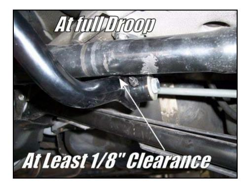
13) Next, fully tighten the jam nut on the end link using an 11/16" open-end wrench. Make sure the heim joint is centered. You may need a flat screw driver or similar tool to hold the heim joint in positioned while you tighten the jam nut.
