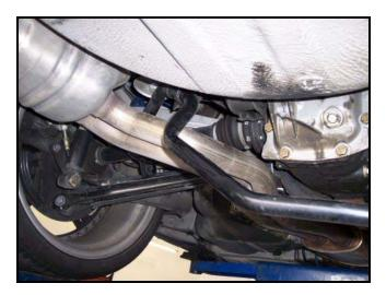
6) Pay close attention to the way the stock end links are mounted to the brackets. These brackets will be used to mount the new end links to the upper cast arms. Remove the stock end links from these brackets and then mount them to the H-Sport end links using the stock hardware. Pay close attention to zerk fitting direction. The lower Zerk Fitting points towards the rear of the car.
