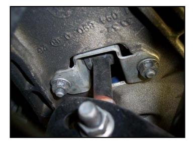
4) Remove the stock bushing brackets on both the driver and passenger sides.
