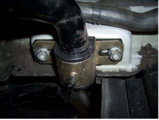
5) Apply grease along the inside surface of your polyurethane bushings and attach them to the Hotchkis bar in the approximate mounting locations. Slip the new brackets over the bushings.
