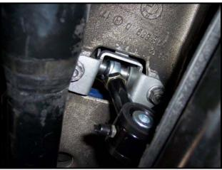
9) Apply grease along the inside surface of your polyurethane bushings. Install the rear bushings onto the bar at the approximate mounting location. Now you may install the Hotchkis rear bar with the H-Sport sticker facing the rear, right side up.
