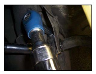
5) The stock rear bar is now free and can be removed as shown below. If you are having clearance problems, you may have to remove the bushings and brackets or even twist the end links forward to remove the bar.
