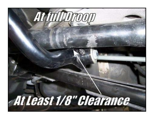
13) Next, fully tighten the jam nut on the end link using an 11/16" open-end wrench. Make sure the heim joint is centered. You may need a flat screw driver or similar tool to hold the heim joint in positioned while you tighten the jam nut.
