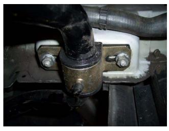
7) Re-install the bracket nuts and tighten. The front uses the larger of the 2 brackets we provide. Then re-install the end link ends and nuts on one of the three available adjustment holes. We suggest the softer adjustment or the holes at the bar's ends.
