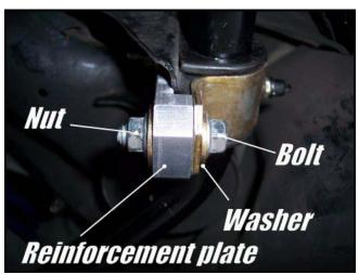
11) Attach the end links to the bar ends (inner hole for more roll resistance and the outer hole {near the ends} for less roll resistance) using the 10mm bolts, nylock nuts and small and large washer. Use the large diameter washer to capture the outboard side of the end link bushing and the smaller washer for the inboard side against the sway bar end.
