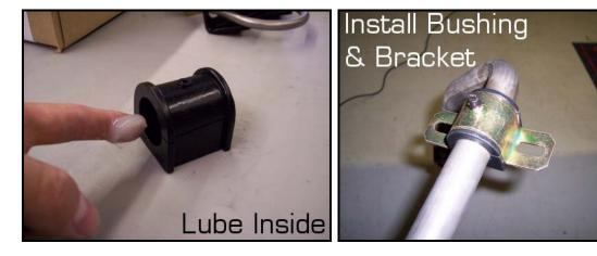
Apply a small amount of anti-seize to the threads of the U-bolts. Next position the axle bracket up against the axle tube. Raise the sway bar up to meet the axle bracket and allow the U-bolts to poke through the bushing bracket. Fasten the assembly together with the provided nut and washer. Do not fully tighten.
