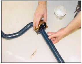
6/ Lift the bar up to the vehicle. The two smaller Hotchkis stickers at the bar's ends should be right-side-up. As you lift the bar up to the mounting points, you must place one mounting plate per side between the bushing and the mounting point. This relocates the bushing out of the stock bushing pocket.
