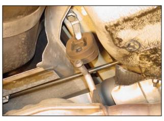
4/ Remove the four bushing bracket nuts and bolts (13mm wrench) attaching the anti-roll bar brackets to the sub-frame and save.
