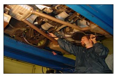
7/ Repeat same pressure to the exhaust and position Hotchkis bar **(without the bushings and brackets)** in the stock location with the "HSport" sticker facing rearward, right side up.
