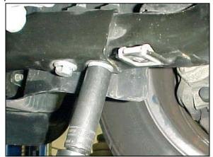
5/ That's it for the sub-frame. Now you must disconnect the lower motor mount. Using the same 16mm socket, or a wrench, remove the horizontal bolt. Then, remove the vertical bolt as shown.
