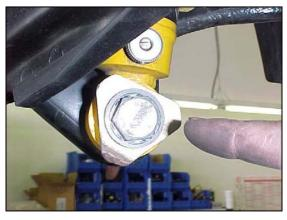
5/ Before removing the sub-frame hardware, remove the four anti roll bar bushing bracket bolts using a 13mm wrench or socket.
