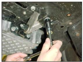
6/ Before removing the front anti roll bar bracket bolts, we highly recommend you remove the four steering rack bolts. Not required but if the sub-frame is pulled down with the rack still attached, this may pop the rubber grommet from the firewall. Removing the four bolts is time consuming but so is reinstalling the grommet – you choose! Use a torx (E
