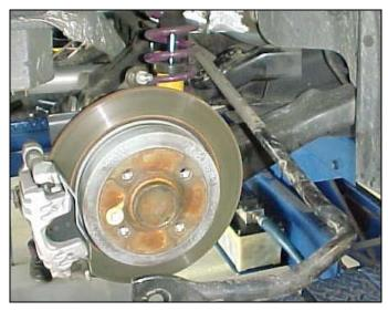
8/ Once the stock bar is out, slide the Hotchkis bar in without the bushings and brackets attached. Once the bar is in the approximate stock location, use the remaining grease on the inside of the rear bushings and slip them over the bar. Then install the supplied bushing brackets with the grease fittings pointing to the outside.
