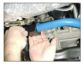
11/ Then, install the larger supplied bushing brackets over the bushings with the grease fittings facing inwards or towards each other.
