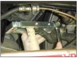
7/ Using the (2), 8mm x 20mm bolts and washers, <u>attach the billet piece to the black bracket (13mm wrench) but DO NOT TIGHTEN</u>. The black bracket is slotted, so use the slots to maneuver the pieces in order to
