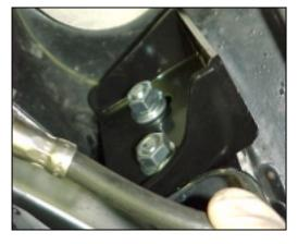
Take one of the supplied billet pieces and remove one of the bolts. This allows you to open the piece and slide over the driver's side toe link. Reattach the bolt and washer (13mm wrench) with the HSport sticker pointing towards the outside of the vehicle and tighten both bolts. You may angle the brace up against the toe link itself to get enough leverage to tighten the bolts
