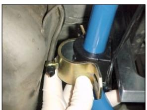
11/ Now, install the last 4 bushing bracket bolts and washers using the 13mm wrench and tighten. Remember, the black bracket is slotted so if all hardware is loose enough, you will be able to thread the bushing bracket bolts through the sub-frame and into the aluminum.
