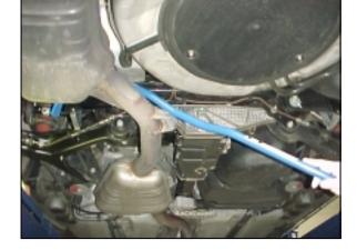
10/ Grease the inner portion of the smaller provided bushings using about one-quarter of the supplied grease pack. With the bar in, at the approx. stock location, install the smaller provided bushings in the approx. stock location. Then, install the bushing brackets with the grease fittings pointing down to the ground.
