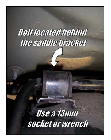
7) Remove the stock sway bar from the vehicle through either side of the differential.
