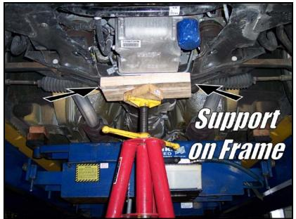
5) You will now disconnect the cradle frame from the vehicle by removing the 2 front bolts and 2 rear bolts using a 16mm and 18mm socket respectively.
