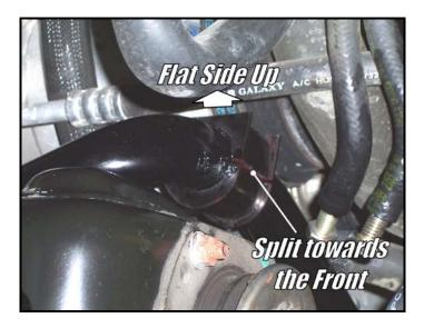
15) Next, grab the Hotchkis saddle bracket and place it over top the bushing. Make sure the zerk grease fittings are pointing toward the front (ignore zerk fitting position in picture). Install the stock nuts using a 13mm socket.
