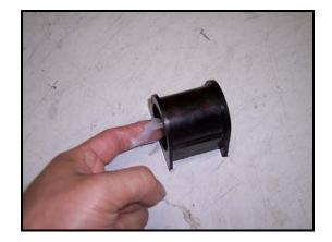
14) Open the bushing and push it over the bar. Make sure the flat side is facing up and the split is in the front.
