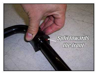
11) Place the stock saddle brackets back onto the Hotchkis polyurethane bushings.
