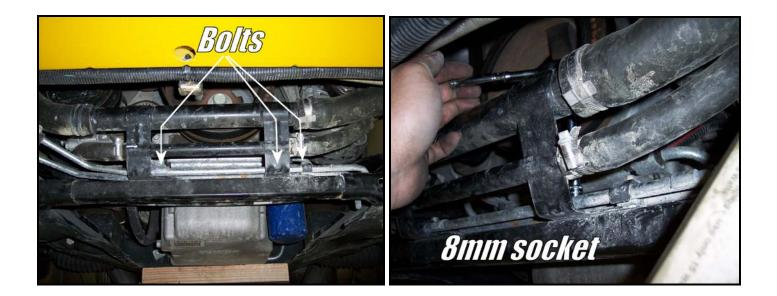
You will notice that the hard transmission lines lay on top of the coolant/transmission line bracket mounts. Make sure to move the transmission lines <u>below</u> the brackets. This will allow the bar to pass through between the coolant lines on top and the transmission lines on the bottom.
