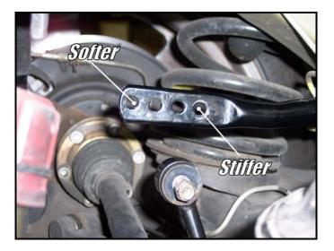
18) You are now finished with the Hotchkis rear sway bar installation! Make sure that all hardware is fully tightened before driving the vehicle.
