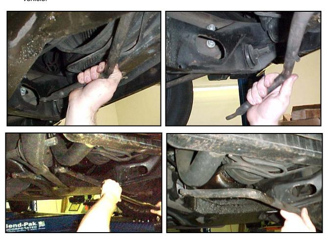
With the stock bar now removed, insert the Hotchkis bar by reversing the previous directions. Make sure the center "hoop" of the bar points down when installing the bar. If the bar is put in backwards, then the bar will contact the balance pulley on the front of the motor. Start by inserting the end of the bar into the round hole on the passenger side of the vehicle frame
