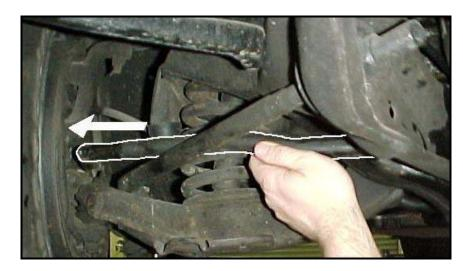
Turn the front wheels to the left until the end of the bar can slide past the rear edge of the brake drum.
