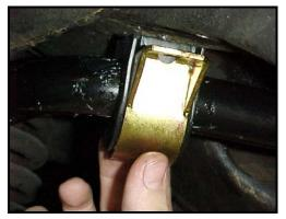
9) With the brackets in place, install the new end links included in the Hotchkis kit at each end of the bar to establish the proper fit of the front bar. The vehicle weight should be on the front wheels to establish the proper ride position of the sway bar in the vehicle.
