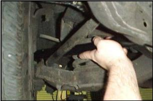
The leading end of the bar should eventually swing into the slot in the frame on the driver's side of the vehicle. The bar will be free moving, but in the proper orientation in the vehicle.
