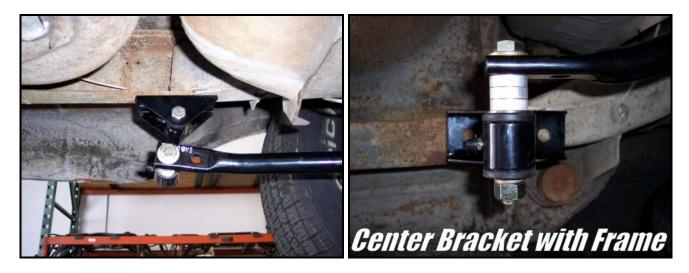
With a marker or scribe, mark the frame for the mounting holes. Drill out the holes to accept a 7/16" bolt. Do this for both sides.
