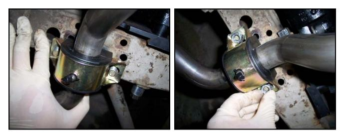
10) You can now fully tighten the endlink nuts & bolts. Tighten endlink until the bushing bulges to the same diameter as the washers.
