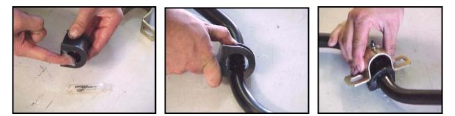
» Hang the sway bar from the u-bolts on the axle. Slide the axle mount bracket over the ends of the u-bolts. Hold the sway bar up into place with the bushing retainer brackets mounted to the axle bracket.
