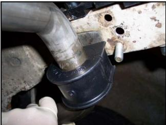
Slide the bushing brackets onto the bushings. Install the remaining washers and nuts from hardware kit #1735. Fully tighten the 4 nuts & bolts.
