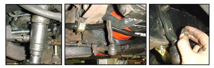
12) Check that all hardware is tight. Cover the grease fittings using the zerk caps provided. Remove the jack stands and move on to installing the rear sway bar!
