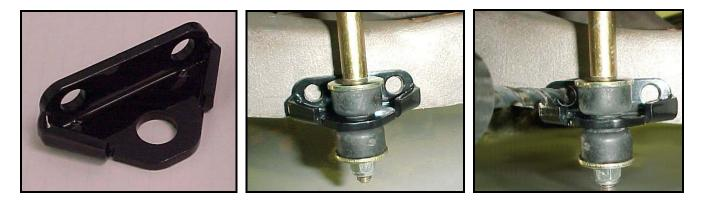
11) With all of the sway bar components in place and tightened down you can re-attach the steering. Push the pitman arm back onto the gearbox in the same position as it was removed. Don't worry if it doesn't slide all the way onto the gear, when you tighten the retaining nut it will move the arm up the shaft. Re-install the bolts holding the idler arm.
