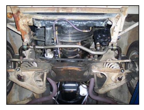
**IMPORTANT!** For proper maintenance the bushings should be greased at least once a year (15,000 miles) or whenever excessive noise occurs. Use only non-lithium based grease. Lithium based grease can wash out with water.
