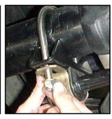
With the bar hanging freely you can slide the u-bolts along the axle until the bar is centered with the vehicle. Tighten down the nuts on the u-bolts to secure the position of the u-bolts and brackets.
