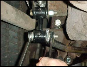
You can also adjust the stiffness of the bar by changing the hole the end link mounts to. The hole nearest to the end of the bar softens the bar stiffness by lengthening the bar. The hole furthest from the end of the bar stiffens the bar by shortening the length of the bar.
