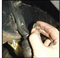
12) Check that all hardware is tight. Cover the grease fittings using the zerk caps provided. Remove the jack stands and move on to installing the rear sway bar!
