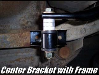
With a marker or scribe, mark the frame for the mounting holes. Drill out the holes to accept a 7/16" bolt. Do this for both sides.
