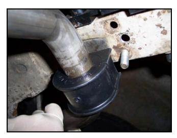
9) Slide the bushing brackets onto the bushings. Install the remaining washers and nuts from hardware kit #1735. Fully tighten the 4 nuts & bolts.
