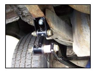
» After all the hardware is loosely in place, fully tighten the hardware starting with the U-bolts. Make sure the U-bolts are facing straight down. Finish off the install by tightening the dogbone hardware. Your Done!!!
