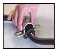
» Hang the sway bar from the u-bolts on the axle. Slide the axle mount bracket over the ends of the u-bolts. Hold the sway bar up into place with the bushing retainer brackets mounted to the axle bracket.
