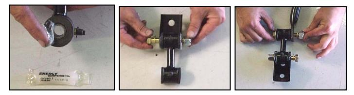
5) Hang the sway bar from the u-bolts on the axle. Slide the axle mount bracket over the ends of the u-bolts. Hold the sway bar up into place with the bushing retainer brackets mounted to the axle bracket.
