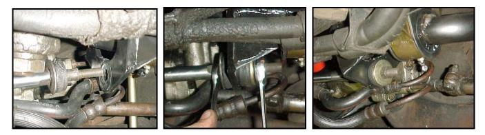
12) Check that all hardware is tight. Cover the grease fittings using the zerk caps provided. Remove the jack stands and move on to installing the rear sway bar!
