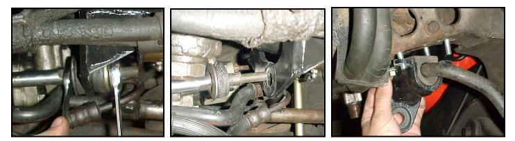
3) Remove the bolts holding the idler arm to the frame. Use a **1-5/16**" **socket or wrench** to remove the retaining nut attaching the pitman arm to the gearbox. Use the pitman arm puller to free the pitman arm from the gearbox.
