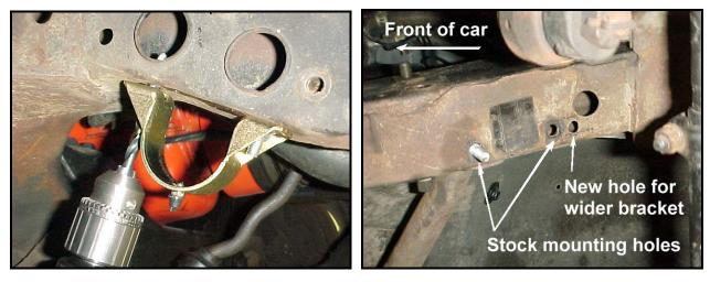
Use the power steering bracket included in the kit and installation pictures to determine which hole must be moved or what holes may need to be added on the driver's side.
