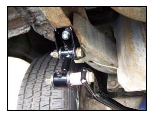
» After all the hardware is loosely in place, fully tighten the hardware starting with the Ubolts. Make sure the U-bolts are facing straight down. Finish off the install by tightening the dogbone hardware. Your Done!!!
