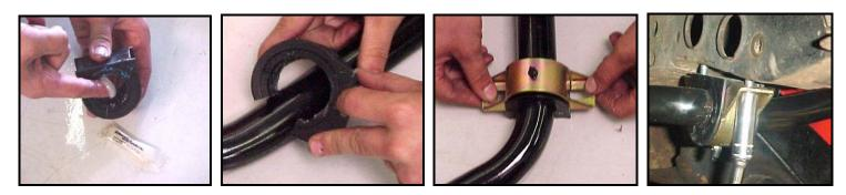
7) With the bar supported on the passenger side you can now slide the power steering bracket over the driver's side end of the bar. The bracket should slide over the bar and line up with the stock mounting holes and the welded stud in the frame.
