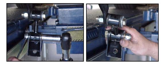
7) With the hardware loosely tightened you can now rotate the bar up, so that the brackets are resting against the frame. Once the brackets are in place use a scribe or similar tool to mark each hole for drilling. Drill out the holes for the brackets to 7/16" diameter. To accurately determine the location of the holes the end links must not be loose enough to move left or right. Make certain the axle is at its normal driving height for an accurate fit.
