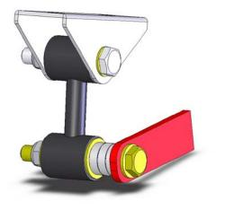
To accurately determine the location of the holes, the end links must NOT be loose enough to move left or right. <u>Make certain the axle is at its normal driving height for an</u> <u>accurate fit.</u> With the hardware lightly tightened, you can now rotate the bar up, so that the brackets are resting against the frame. Make sure both clevis brackets lay in the center of the frame. Position the clevis bracket onto the frame so that it will be possible to use either hole on the sway bar end.
