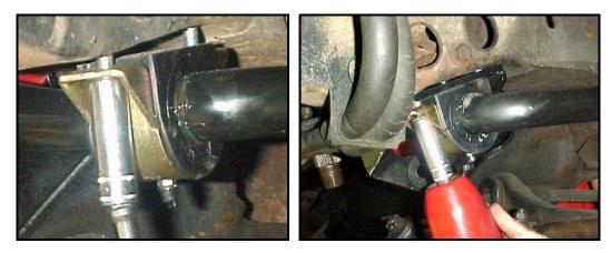
The driver's side bracket mounts inside of the power steering bracket included with the Hotchkis kit. Slide the retainer bracket into place over the bolts and tighten the bracket into place.
