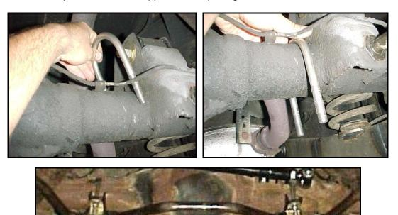
3) Use the grease pack provided to apply a heavy coat of grease to the inside of the sway bar bushings. Place the bushings over the bar. Push the brackets onto the sway bar bushings.
