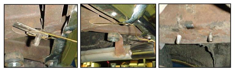
9) Rotate the sway bar so that you can bolt the brackets up to the stud plate in the frame using the 7/16" hardware from kit #T1719. You will only be using four of the nuts and the four smaller washers on the studs. The four additional nuts and washers are extra hardware not used on this kit and may be discarded. Tighten the nuts on the brackets and the end link hardware. Torque the end link hardware to 30ft/lbs.
