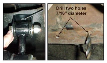
8) Once the holes are drilled, use a coat hanger to loop around one stud on the retainer bracket. Slide the bracket in through the rear end of the frame until the studs fall through the holes. Hold one stud and push the other stud back through the hole to slide the coat hanger loop off the stud.
