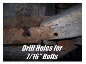
» Once the holes are drilled, grab a 7/16" x 1.25" bolt (longer) and a 7/16" washer. Using a telescoping magnet wand, fish the bolt and washer through the box tubing and set the bolt into it's drilled out hole.
