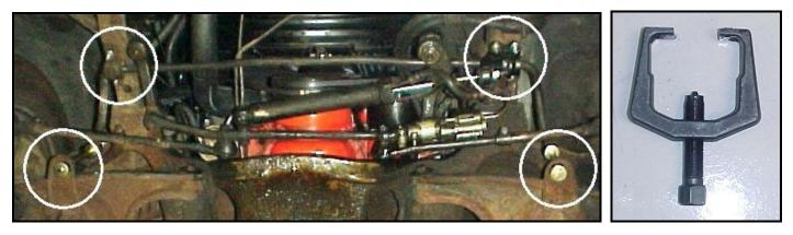
The car shown above has power steering and a sway bar factory installed. Owners of cars without a factory sway bar should note the position of the brackets and end link mounts, as you will be adding all of these at a later time.
