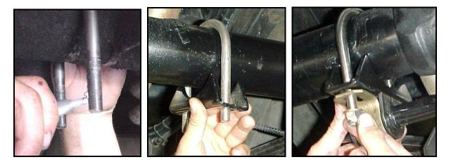
With the bar hanging freely you can slide the u-bolts along the axle until the bar is centered with the vehicle. Tighten down the nuts on the u-bolts to secure the position of the u-bolts and brackets.
