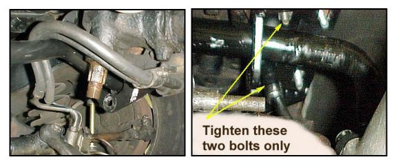
Route the power steering lines over the sway bar!
