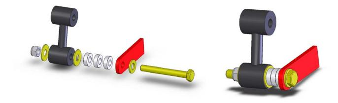
» Install the Clevis Bracket onto the dogbone endlink. Lightly tighten.
