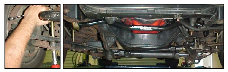
For cars without a stock front bar, you will have to connect the end links to the sway bar. Attach the end link mount bracket included with the kit to the end links and tighten. Rotate the full assembly into position against the lower a-arm and drill the mounting holes in the arm. Use the 10mm bolts from hardware kit #T1711 to secure the brackets.
