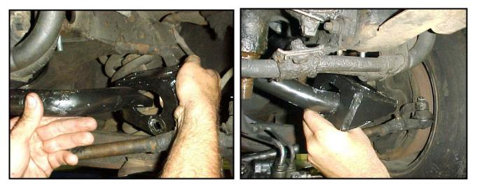
Tighten the hardware on the inside edge of the bracket nearest to the hole that the bar passes through.
