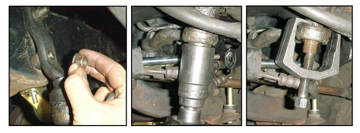
Note the position of the gearbox teeth and pitman arm to maintain proper steering when re-installing the pitman arm in a later step!
