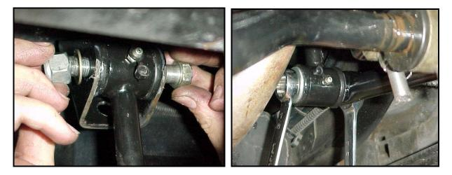
**WARNING:** Check the end link clearance to the bracket hardware. If the hardware contacts the end link it can wear a hole though the end link as the bar pivots during use. You will not be able to install the bar if the stud plate makes contact with the end link.
