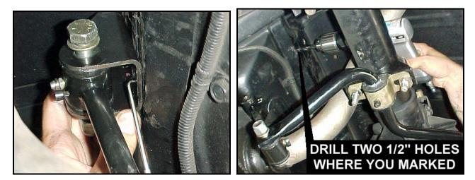
12) Drop the stud plate in from the passenger compartment through the holes. **Place one of the large washers provided over the lower stud on the plate**. This will act as a shim. It is also *suggested* to apply a ring of silicone gasket sealer to the edges of the holes and the stud plate to act as a water sealant.
