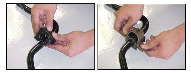
6) Grease the outsides of the bushings at each end on the 'dog-bone' end links. Use the long (3") bolts from **hardware kit #T1712** to connect the end links to the inside of the sway bar. *Make certain the larger diameter washer is up against the bushing side and the smaller washer is up against the sway bar side.* This will prevent the bolt from pulling through the bushing over time. 'Hand tighten' the hardware only at this step. *Leave the end link loose enough to rotate.*
