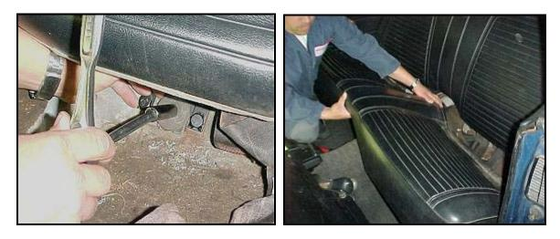
**IMPORTANT:** For proper maintenance grease the bushings at least once a year (15,000 miles) or whenever excessive noise occurs. Use a non-lithium based grease only! Lithium grease can dissolve with water and should not be used.
