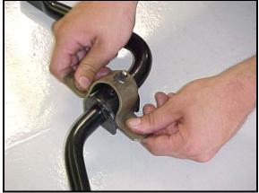
Grease the outsides of the bushings at each end on the 'dog-bone' end links. Use the long (3") bolts from **hardware kit #T1712** to connect the end links to the inside of the sway bar. *Make certain the larger diameter washer is up against the bushing side and the smaller washer is up against the sway bar side*. This will prevent the bolt from pulling through the bushing over time. 'Hand tighten' the hardware only at this step. *Leave the end link loose enough to rotate*.
