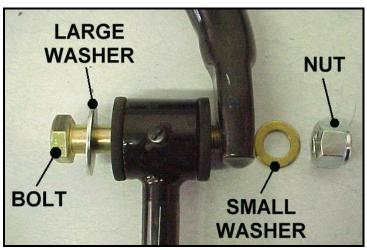
7) Use the shorter length bolts (2-3/4") from **hardware kit #T1712** to attach the triangular bracket to the end links. *The larger end of the bracket should be closer to the ground when installed.* Loosely start the hardware so that the assembly can rotate freely.
