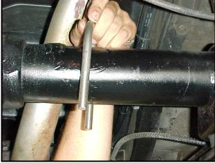
9) Lift the bar assembly into place under the rear of the car with the arms of the bar pointing forward. Use the axle mount brackets provided to hang the sway bar loosely from the axle. Slide the u-bolts as necessary to center the sway bar on the axle.
