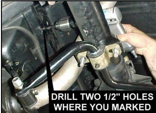
Drop the stud plate in from the passenger compartment through the holes. **Place one of the large washers provided over the lower stud on the plate**. This will act as a shim. It is also *suggested* to apply a ring of silicone gasket sealer to the edges of the holes and the stud plate to act as a water sealant.
