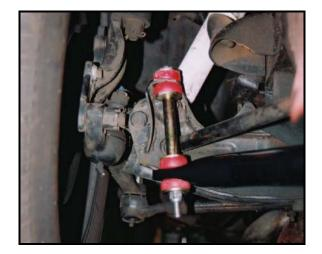
6. Once the end links are attached, install the bushings and brackets to the bar. Make sure to apply the included silicon grease. You will also need to install the new Hotchkis bushing retainer bracket onto the bushing bracket as shown in the picture. Attach the driver and passenger side D-Shaped bushing & bracket and position them as outboard as possible.
