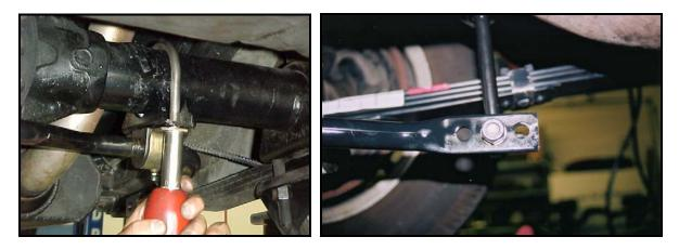
In the above picture the hole to the left is stiffer and the hole to the right is softer. Check that all attaching hardware is tight. Make certain the zerk fitting caps are covering the grease fittings. Lower the car from the jack stands and you're done!
