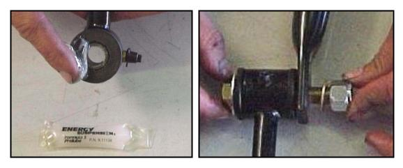
Use the grease pack to also apply a thick coat of grease to the insides of the sway bar bushings. Place the bushings over the bar with the split of the bushing facing towards the rear. Install the bushing retainer brackets over the bushings.
