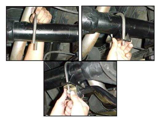
Use the tube of anti-seize included with the kit to apply a small amount to each set of threads on the u-bolt. **DO NOT** tighten the nylock nuts without using anti-seize! You could ruin the nuts or snap the u-bolt without it.
