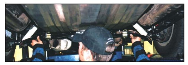
Place the u-bolts over the rear axle. Slide the axle brackets over the ends of the u-bolts with the curved side up against the axle. Rotate the bar into position and slide the bushing retainer brackets over the ends of the u-bolts. Start the nylock nuts onto the ends of the u-bolts to loosely hold the bar to the axle.
