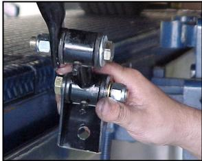
8) Rotate the bar upwards, so that the brackets are resting against the frame. Once the brackets are in place use a scribe or some other tool to mark the center of each hole for drilling.
