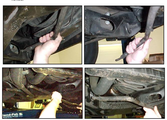
With the stock bar now removed, insert the Hotchkis bar by reversing the previous directions. Make sure the center "hoop" of the bar points down when installing the bar. If the bar is put in backwards, then the bar will contact the balance pulley on the front of the motor. Start by inserting the end of the bar into the round hole on the passenger side of the vehicle frame
