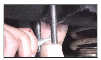
Use the anti-seize provided with the u-bolts to lubricate the threads. Failure to lubricate the threads can destroy the nuts and possibly break the u-bolt or seize the nut in place when tightened.
