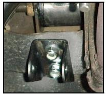
11) Re-attach the end links to the brackets and tighten the hardware into place. Torque the end link hardware to 80 ft/lbs.
