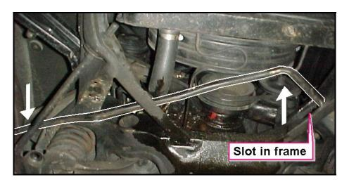
5) The end of the bar on the driver's side should now be free. Pull the end of the bar towards the front bumper and rotate as necessary to remove the bar from the vehicle. <u>Do not</u> straighten the front wheels at this time. They should still be turned slightly towards the driver's side of the vehicle.
