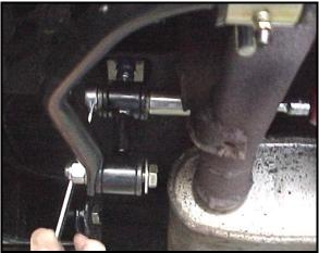
12) Check that all hardware is tight. Use the caps provided to cover the zerk fittings and you're done installing the Hotchkis rear sway bar!
