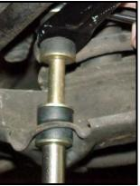
13) Re-check all hardware for tightness. Cover the zerk fittings in the brackets with the grease caps that came attached to the brackets. You are finished with the front sway bar installation
