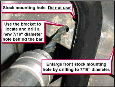
11) Use the 3/8" bolts from **hardware kit #1735** to attach the Hotchkis bar. Drop the bolts down through the drilled out holes in the frame. Start the washers and nylock nuts onto the ends of the bolts. You will use only four of each nut, washer and bolt. <u>DO NOT THROW THE EXTRA HARDWARE AWAY</u>, as it is used for the rear sway bar. Torque the hardware to 35 ft/lbs.
