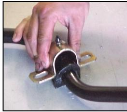
4) Use the grease provided to apply a heavy coat of grease to the sides of the bushings on the "dog bone" end links. Attach the mounting brackets to the end links using **hardware kit #T1712**. Attach the other end of the links to the sway bar. Leave the attaching hardware loose.
