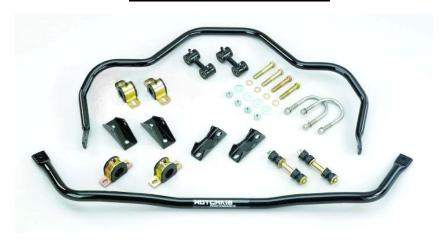
This installation will require drilling new mounting holes for both the front and rear sway bars. *Please read instructions carefully to avoid unnecessary drilling.*
