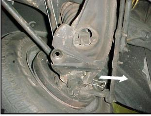
4) Move the sway bar end towards the rear on the passenger side of the vehicle until the opposite end of the bar clears the slot in the frame on the driver's side.
