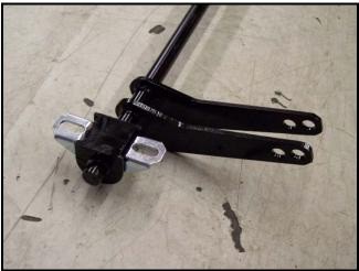
Position the sway bar onto the truck as shown. The sway bar lever arms point towards the rear. Use the hardware from bag #17118-1 to mount the bushing bracket to the frame. The longer bolts (1.25") are for the front hole and the shorter bolts (1") mount the rear holes. Center the bracket so that the holes are in the middle of the bracket slots. Fully tighten the bolts.
