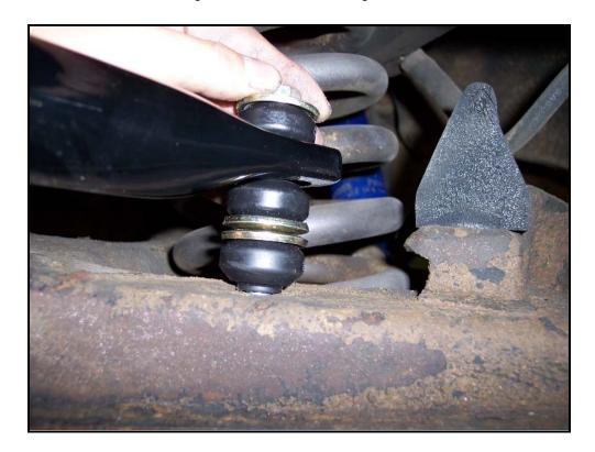
Insert the bolt through the a-arm and install the smaller diameter bushing and a small washer from the bottom of the arm. Tighten everything with the included nylock nut.
