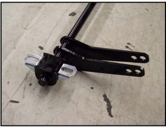
Position the sway bar onto the truck as shown. The sway bar lever arms point towards the rear. Use the hardware from bag #17118-1 to mount the bushing bracket to the frame. The longer bolts (1.25") are for the front hole and the shorter bolts (1") mount the rear holes. Center the bracket so that the holes are in the middle of the bracket slots. Fully tighten the bolts.
