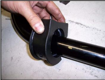
Slide the bushing brackets onto the bushings as shown below.
