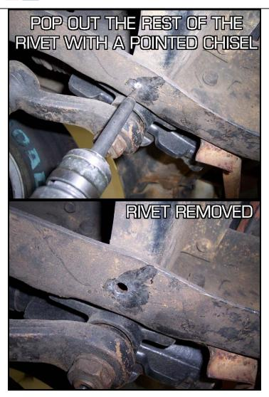
Once the holes are clear, grab the  $3/8" \times 1.5"$  hex bolts & washers from the "front" hardware bag and insert them into the rivet holes facing down.
