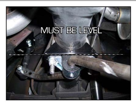
3R Loosely attach dog bones to middle hole on sway bar, and to frame brackets. Use hardware kit T1712.
