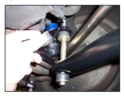
With end links attached, loosely install the sway bar bushings, brackets, and frame mounts to the inboard side of the sway bar centering rings. Lift sway bar, and position brackets and frame mounts evenly side to side, as well as fore & aft, to keep end links vertical. Clean and prep the surface of frame, and tack weld into position. See following steps.
