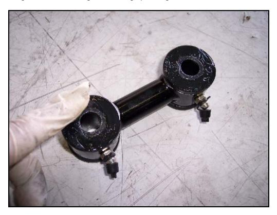
Install the line bracket onto the long bolt and install a washer and nut. Do not fully tighten at this time. (hardware kit **#1757**)
