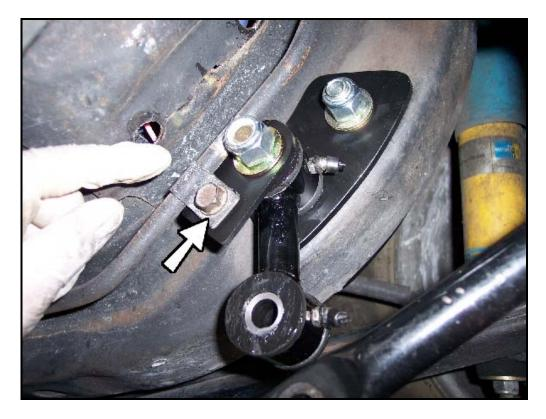
Fully tighten both short and long bolts completely.
