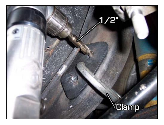
Remove the vise clamp and insert 1 short bolt w/ washer and 1 long bolt w/ washer from the outside of the frame rail. (hardware kit **#1757**) Make sure to add the other reinforcement plate to the outside before you insert the bolts through the frame.
