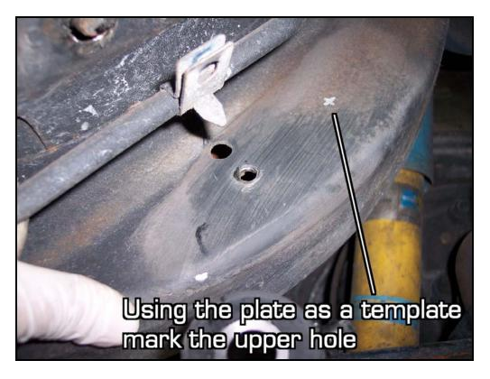
Drill out the <sup>3</sup>/<sub>4</sub>" hole only on the inner side of the frame rail. Do not drill through both walls of the frame rail. We found that a unibit works best.
