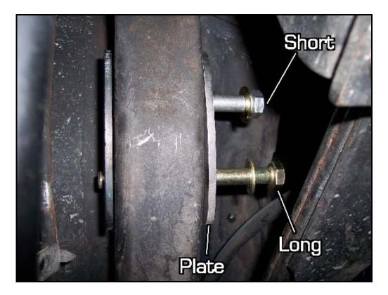
Install a washer and a nut to the top (shorter) bolt. Do not fully tighten this bolt at this time. (hardware kit **#1757**)
