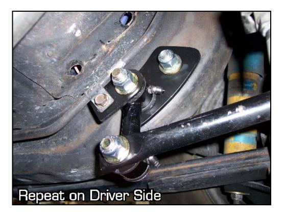
Once the passenger side is completely mounted together, you can now figure out where the other frame rail reinforcement plate goes on the driver side. Mock up the driver side dog bone end link onto the sway bar and mark where the bottom hole should be. Again, use the reinforcement plate as guide to mark the upper hole. Drill the holes in the same manner as before.
