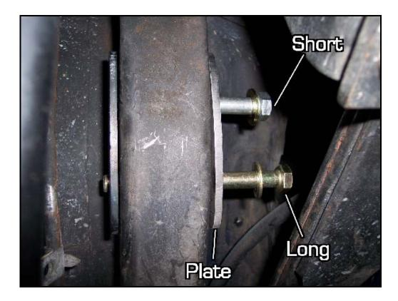
Install a washer and a nut to the top (shorter) bolt. Do not fully tighten this bolt at this time. (hardware kit **#1757**)
