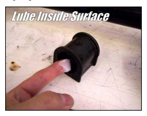
3R. Install the bushings on the bar. (5) Place the bracket over top of the bushing. (6)
