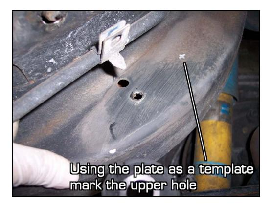
Drill out the ¾" hole only on the inner side of the frame rail. Do not drill through both walls of the frame rail. We found that a unibit works best.
