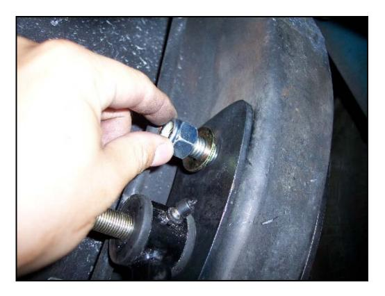
Grease up your new dog bone end links with the provided grease. Install the dog bone on the bottom (longer bolt) with the grease fittings pointing rearward.
