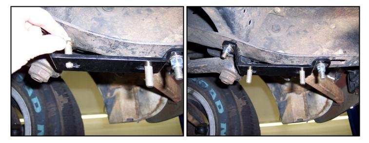
You can now fully tighten the frame bolts at this time.
