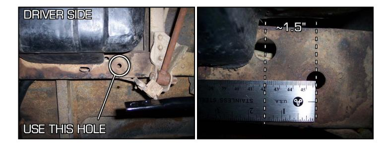
Go to the passenger side frame rail and measure the same dimension and mark the frame with a paint pen. Drill out the hole using a 7/16'' drill bit.
