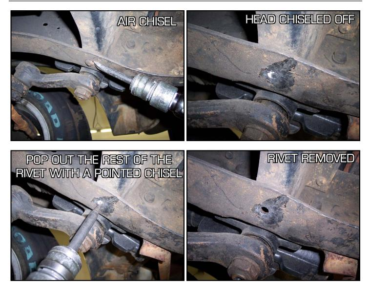
Once the holes are clear, grab the  $3/8" \times 1.5"$  hex bolts & washers from the "front" hardware bag and insert them into the rivet holes facing down.
