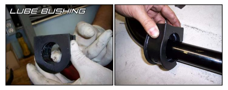
Slide the bushing brackets onto the bushings as shown below.
