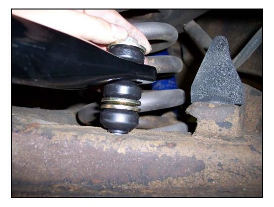
Insert the bolt through the a-arm and install the smaller diameter bushing and a small washer from the bottom of the arm. Tighten everything with the included nylock nut.
